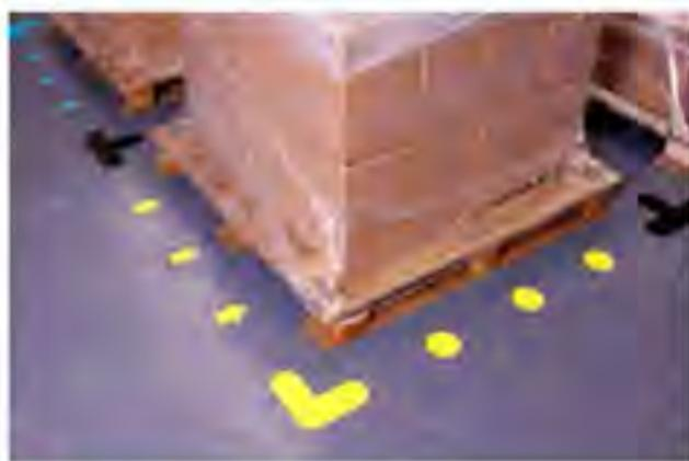
Multi-pallet bays help logistics planning - the durable components can withstand sustained fork-lift traffic
